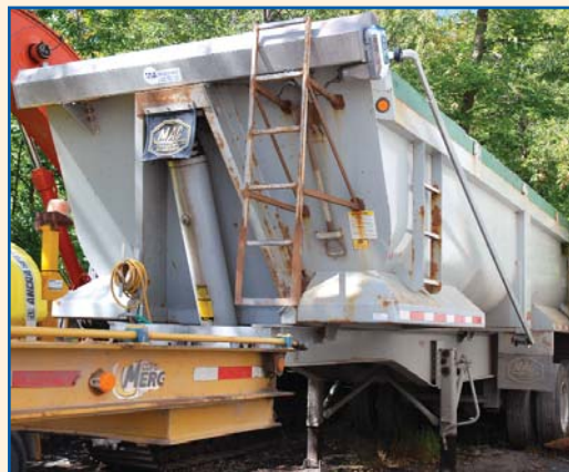
MAC T/A END DUMP TRAILER
